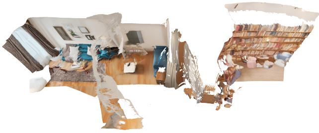
Figure 2: A birds-eye view of two meshes that failed to blend due to the lack of geometric guidance and context throughout the iterative mesh completion process.
